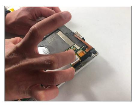
Remove the motherboard from the outer case.
