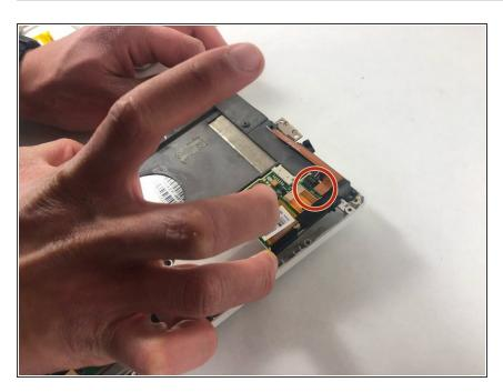
Remove the motherboard from the outer case.
