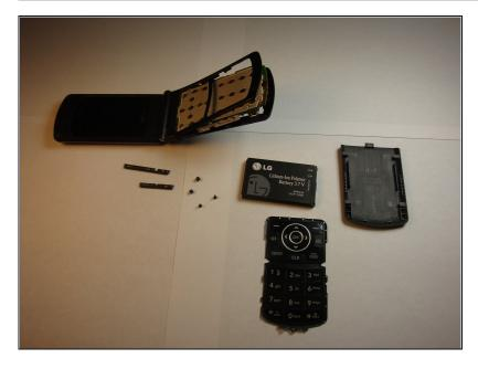
In order to disassemble the phone, you will need to follow the <u>General Disassembly LG</u> <u>VX8560</u> first.
