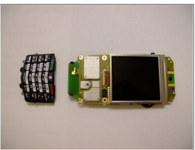
Use a plastic opening tool to lift up the two black clips indicated in the picture.
