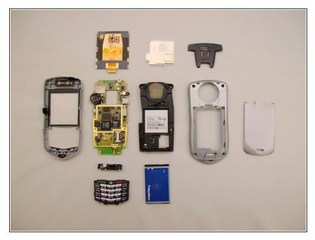
Here are all the parts of your Blackberry 7105t, fully disassembled.
