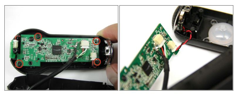
Remove the four 6mm Phillips #0 screws connecting the motherboard and front cover.
