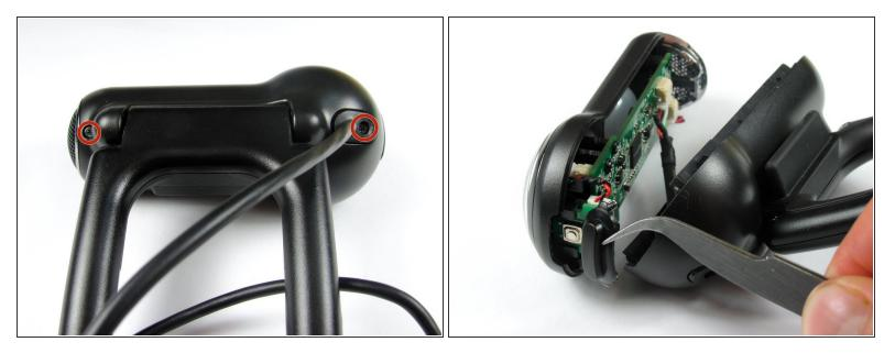
• Remove the two 8 mm Phillips #0 screws on the back cover.
