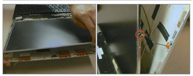
• Use a Phillips #000 to unscrew the one 2.8 mm fine thread screw holding the wire connected to the right face of the LCD.
