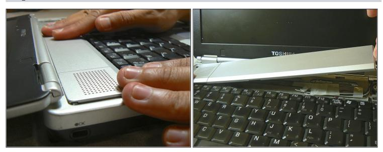
• Remove the rest of the cover by sliding it to the right and lifting the right edge.
