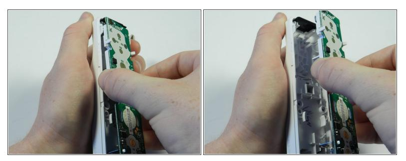
• Grasp the edges of the motherboard and pull it straight away from the case.
