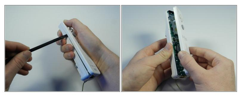
• With the flat end of a spudger, gently apply pressure to the tabs located on left side of the controller.
