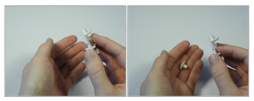
Gently push the rubber button out of the plastic housing.
