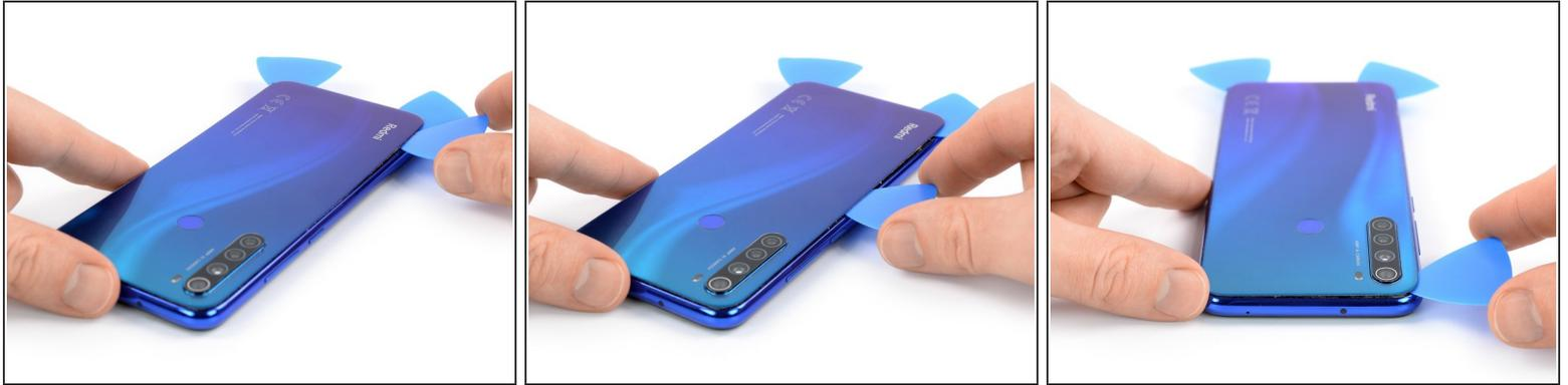
**i** If the adhesive becomes hard to cut, it has most likely cooled down. [Use your iOpener](#) for one to two minutes to reheat it.
