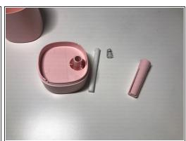
Remove the cotton swab and spring from inside the humidifier.
