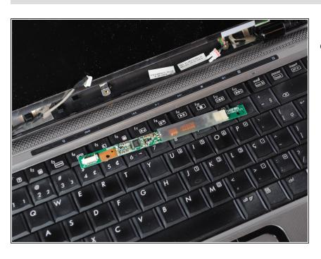
Remove the inverter from the device.
