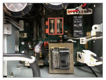
There are two fuses on the PS (Power Supply) Board, which is underneath the AC Board. Check the fuses for continuity as before.
