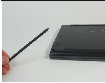
• Remove stylus from the lower left corner of the back panel.
