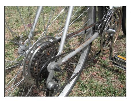
Shift the bike's rear derailleur onto the innermost gear.
