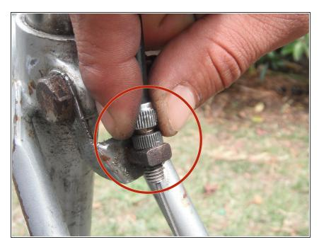
Afterwards, you can fine-tune the adjustment by tightening or loosening the barrel adjuster located about 7 inches above the brake levers.
