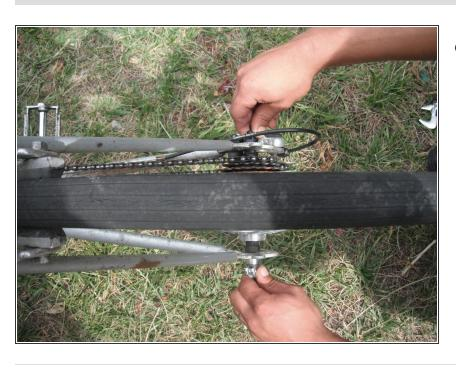
Now that the axle is placed correctly, re-tighten the axle and reapply the quick-release as shown in Step 1.
