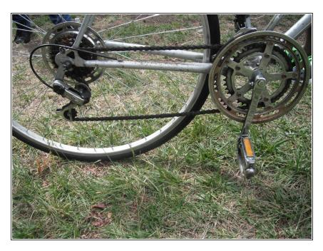
Shift the rear derailleur into its outermost gear, and the front derailleur into its outer gear.
