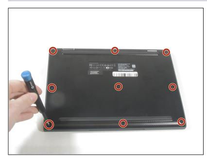
• Remove nine 6 mm screws from the bottom cover of the laptop using a Phillips #0 screwdriver.
