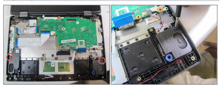
• Remove the two 4 mm screws (one on each speaker) using a Phillips #00 screwdriver.
