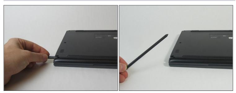
• Remove stylus from the lower left corner of the back panel.
