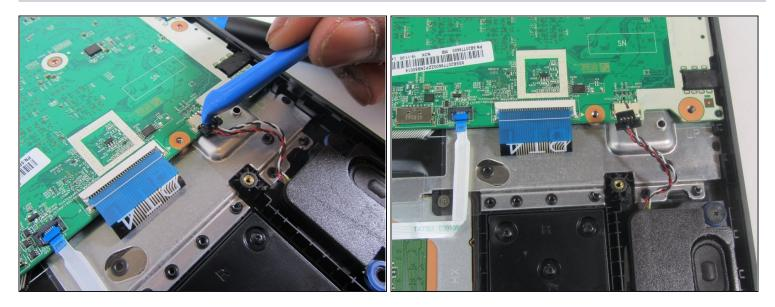
• Use the iFixit opening tool to detach the right speaker cable from the motherboard.
