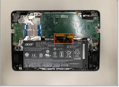
• Once the back cover is removed, you will see that the battery is only held in place with a piece of ESD Tape. Using a set of tweezers, carefully peel away the tape from one end.
