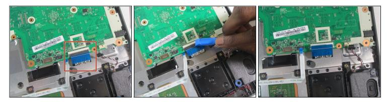
Using an iFixit opening tool, detach the keyboard cable from the motherboard.
