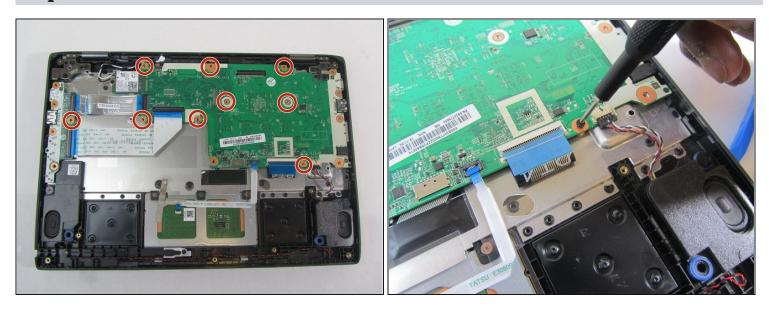
• Remove the nine 4 mm screws from the motherboard using a Phillips #00 screwdriver.
