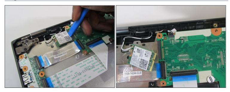
• Disconnect the Wi-Fi card from the motherboard using an iFixit opening tool.
