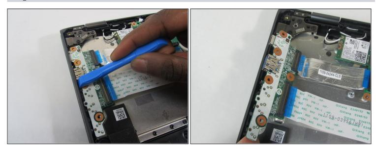
• Gently remove the USB port from the side housing using an iFixit opening tool.
