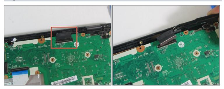
• Using tweezers, disconnect the black cable from the motherboard.
