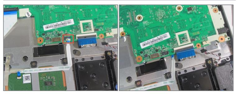
• Using an iFixit opening tool, detach the track pad connector from the motherboard.
