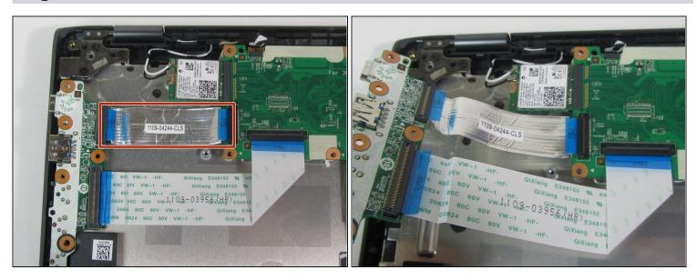
• Gently peel the metal strip away from the metal backing.
