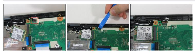
• Using an iFixit opening tool, disconnect the camera cable.
