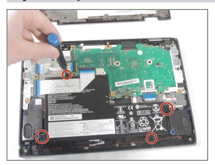
Remove the four 4 mm Phillips #00 screws holding the battery in.
