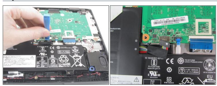
• Use the iFixit opening tool to unplug the battery from the motherboard.
