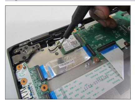
Remove the single 3 mm screw that holds the Wi-Fi card in place using a Phillips #00 screwdriver.
