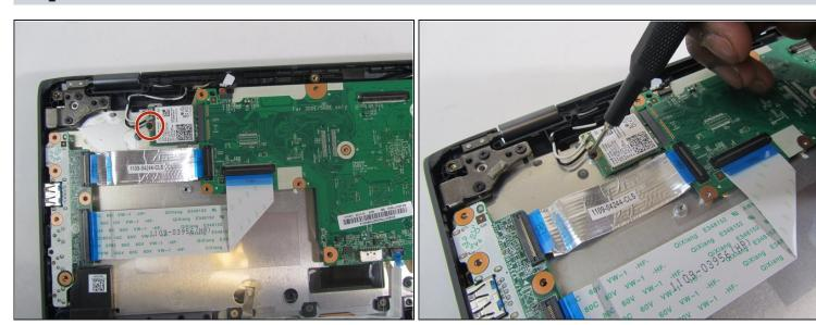
• Remove the single 2 mm screw from the Wi-Fi card using a Phillips #00 screwdriver.
