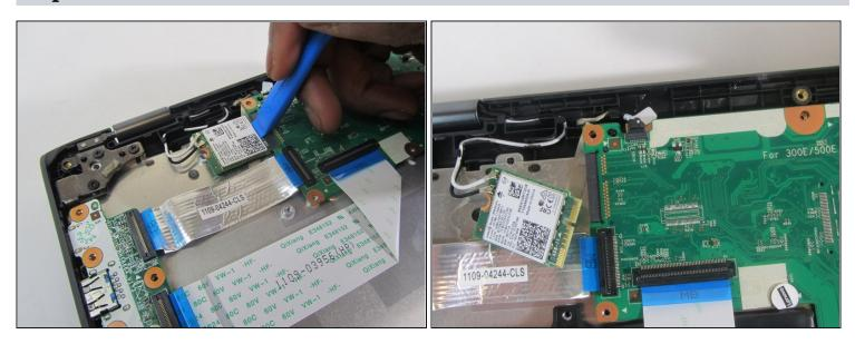
• Detach the Wi-Fi card from the motherboard using an iFixit opening tool.
