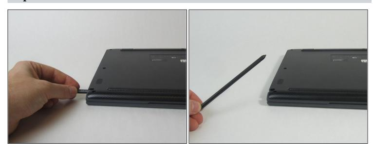
• Remove stylus from the lower left corner of the back panel.
