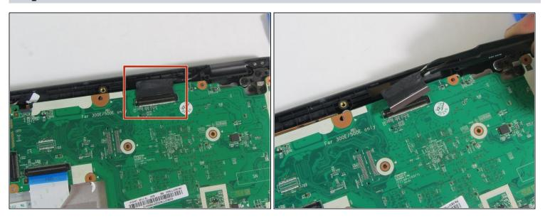
• Using <u>tweezers</u>, disconnect the black cable from the motherboard.
