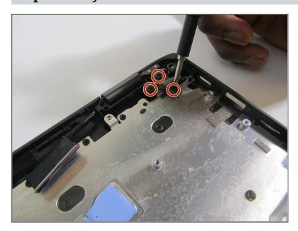
Remove the three 5 mm screws (six total) from each hinge using a Phillips #0 screwdriver.
