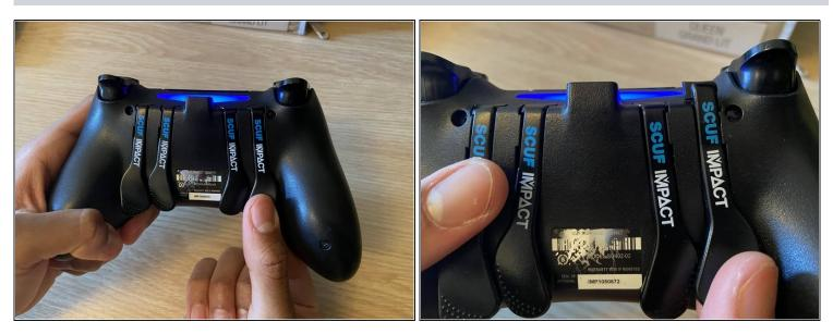
• Push the back button upward until the top piece slides out.
