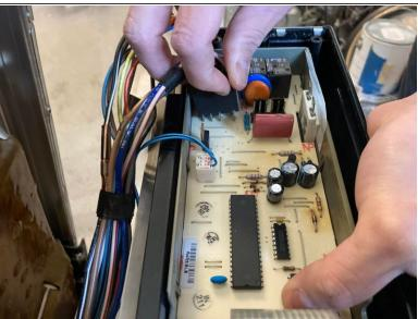
Reconnect the black connector wires to the new electronic control board.
