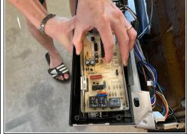
Detach the white and gray ribbon cable attached to the black connector.
