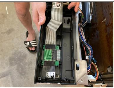
Use your hands to pull the electronic control board out the mounting slots.
