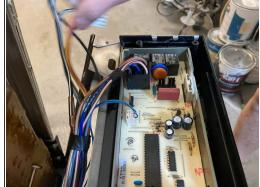
Remove the white rectangular connector that has six colored wires connected to it.
