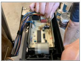
Reconnect the two white outer connector wires to the new electronic control board.
