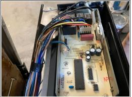
Reconnect the white rectangular connector with six wires to the new electronic control board.
