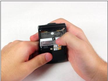
• Remove the battery by pushing down on the top and pulling it away from the phone.
