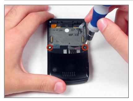
Unscrew the two 5mm T6 Torx screws form the phone.
