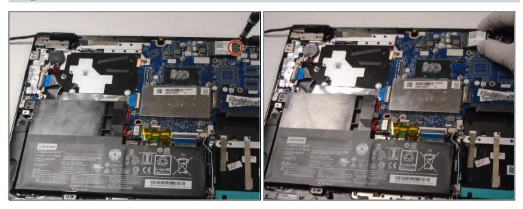
• Use a Phillips #00 screwdriver to remove the single screw securing the Wi-Fi card.
