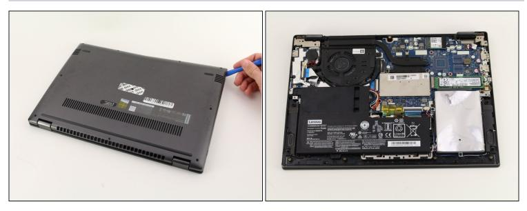
• Use the plastic opening tool to lift up and remove the casing.
