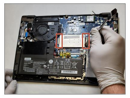
• Use a spudger to gently bend down the locking tabs on the RAM casing.
