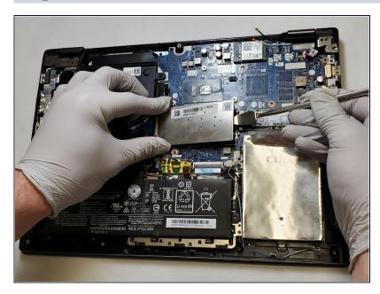
• Use a spudger to gently lift the RAM casing, then lift it up and off.
