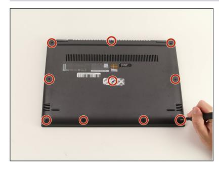
Remove all ten 6.6 mm screws with a Phillips #00 screwdriver.
