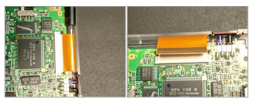
Using a spudger, screwdriver or other long thin object, gently pull the ribbon cable out of the bracket.
