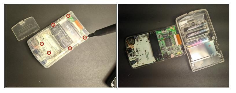
Using a Y1 screwdriver, remove the six screws on the back of the device.
