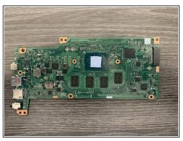
Once we have the hinges free, all we have to do is remove the three screws and lift the motherboard out.
