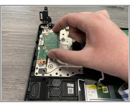
There are three 4.65 mm screws holding the daughterboard in place. Two of those screws hold a screen hinge in place. Once the screws are removed, you are going to need to lift the hinge to remove the board.
