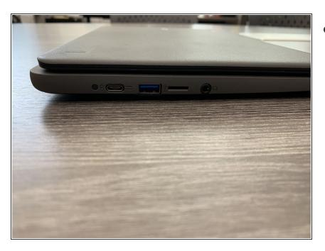
This unit comes with two regular USB-C ports and two 3.0 USB-A ports. So there is at least one port on the left and right-hand sides of the device. However, the lefthand side of the unit has a standard 3.5 mm headphone jack and a micro SD card slot for storage expansion.
