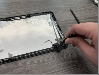
• It's also worth pointing out that the screen hinges can be removed. The only thing holding them in place are 3 Phillips head screws.
