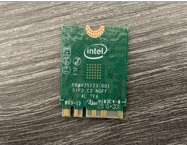
After removing the card, we can see that IEEE 802.11a/b/g/n/ac wireless connectivity is provided by Intel's "Dual Band Wireless-AC 7265"
