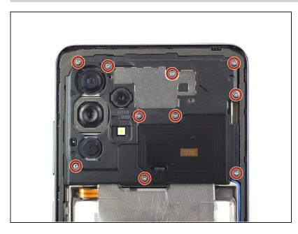
Use a Phillips screwdriver to remove the ten 4.4 mm-long screws securing the motherboard cover.
