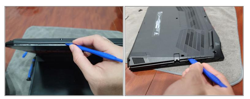
Slide an iFixit opening tool into the front lip of the laptop and slowly move your way around the chassis.
