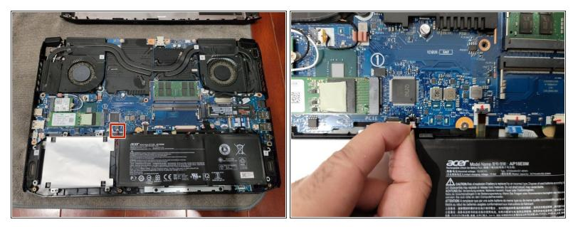
• Disconnect the battery by either using the iFixit opening tool or your fingers.
