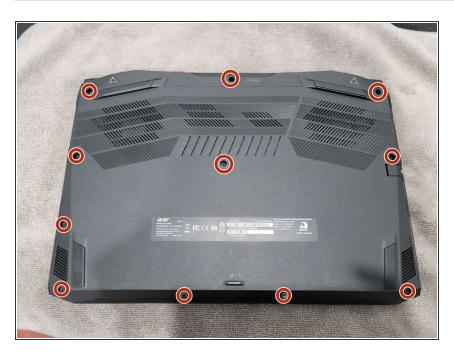
Remove eleven screws from the bottom case of the laptop using a Phillips #00 screwdriver.
