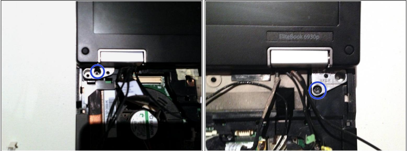
**!** The display assembly will be unsupported when the following screws are removed. To prevent damage support the display before removing the screws.
