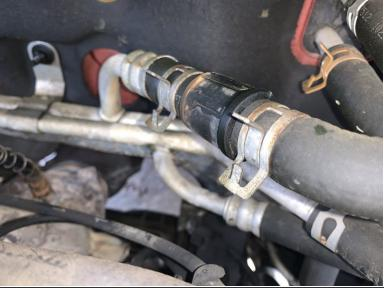
• Locate the regulator valve under the windshield wiper assembly, just in front of the firewall.
