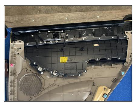
After the door panel is fully disconnected, it should be set on a flat surface with the screw side face up.
