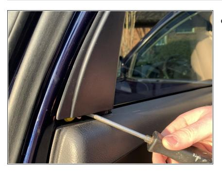
After removing all four screws, remove the small triangular plastic piece above the door panel by using a flat head screwdriver and prying the piece up.
