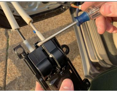
After removing the electrical connection, the locking mechanism of the door handle must be removed. This can be done by pressing the tab located on the back of the door handle mechanism.
