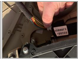
Once the door panel is completely off, the electrical connection in the door frame must be disconnected and removed.
