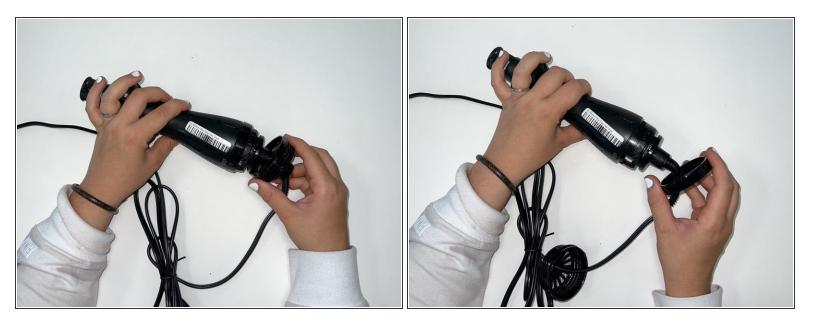
• Next, slide down the air inlet and the setting dial to reveal the 11mm screws on each side of the handle at the bottom of the hair dryer.
