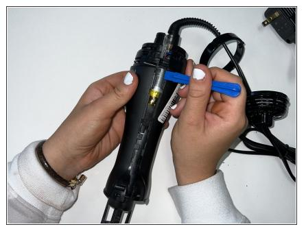
• Place the iFixit opening tool along the seams of the handle and pry the two pieces apart.
