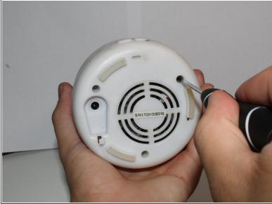
• With a Phillips #1 screwdriver, remove the three 10 mm screws on the bottom of the diffuser.
