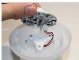
To separate the board from the water tank, unscrew the three Phillips #1 10 mm screws securing the board.
