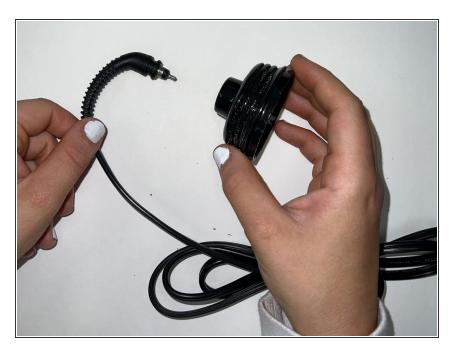
Remove the air inlet by sliding it completely off of the wire.
