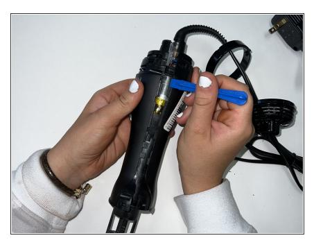
Place the iFixit opening tool along the seams of the handle and pry the two pieces apart.
