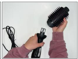
Remove the barrel by twisting and pulling it away from the handle of the dryer.
