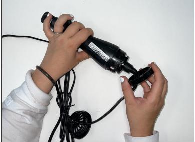
Next, slide down the air inlet and the setting dial to reveal the 11mm screws on each side of the handle at the bottom of the hair dryer.
