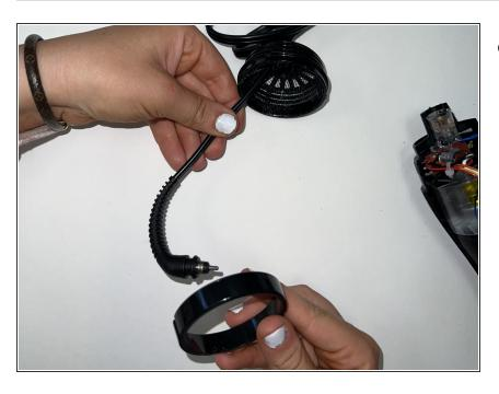
Once the cord is disconnected from the handle, you should be able to slide the dial setting off completely and free it from the cord.
