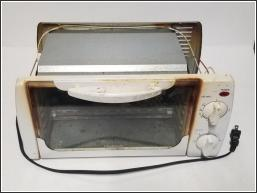
With the appliance facing you, remove the top cover of the toaster oven to access the timer location.
