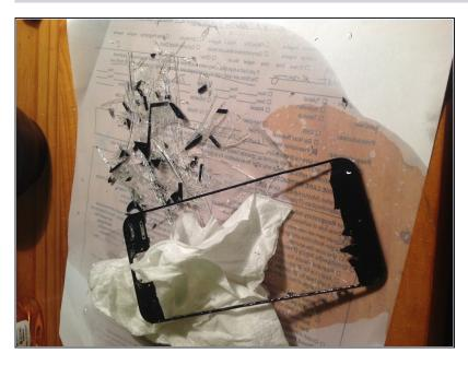
Clean the rest of the glass and goo off of the frame. I used the same heat and adhesive remover method, but a touch more heat here is okay.
