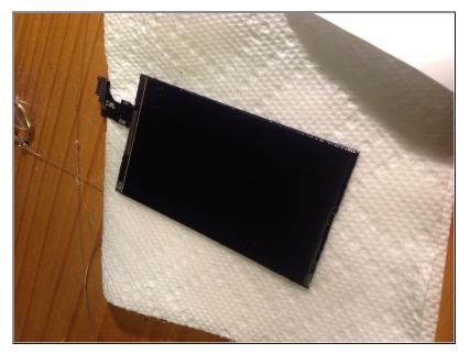
• After all the glass is removed from the LCD, gently soak it down in adhesive remover and use your fingers to get rid of the rest of the goo
