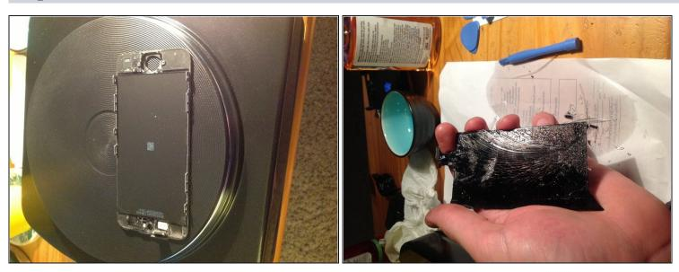
• Using a hot plate (cooktop) and a temp gun heat up the LCD to about 150-160 degrees. I also soaked the display in Duck Brand adhesive remover. Working a few pieces of glass at a time soaking and heating. I used a small flat head, plastic pry and a high guitar string to remove all the glass from the LCD. Be careful not to twist the LCD assembly.
