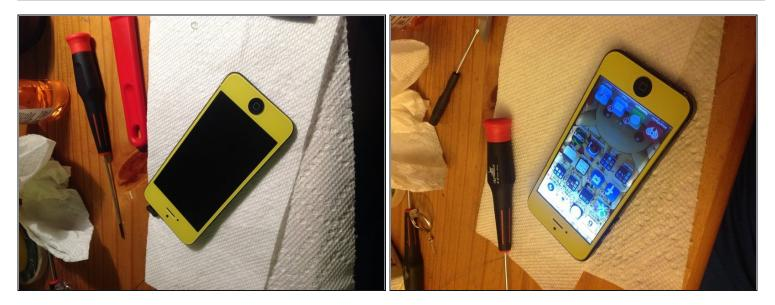
• Attach the new glass to the frame and LCD. I only attached the glass to the frame on mine for various reasons. Others recommend using an optically clear adhesive to attach the new glass to the LCD directly. Then reassemble the display and install.
