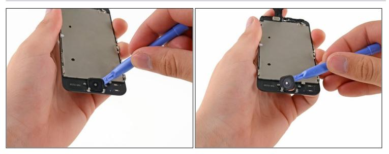
• Use a plastic opening tool to pry the home button up from the display assembly.
