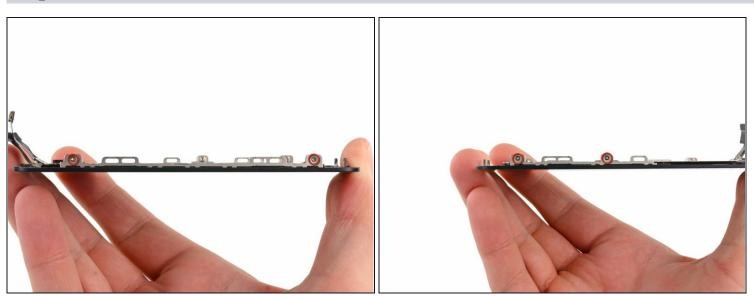
• Remove two 1.2 mm Phillips screws from each side of the LCD frame (four total).
