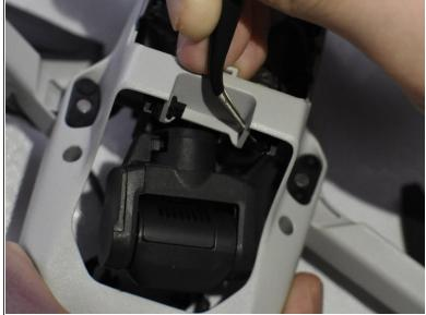
Use the tweezers to pull the four rubber camera holsters off of the body.
