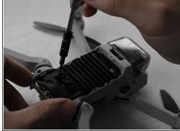
Remove the three 3mm J000 screws on the black plate.
