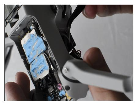
Using the ESD Safe Blunt Nose Tweezers, pull the two gray wires through the drone chassis to the other side.
