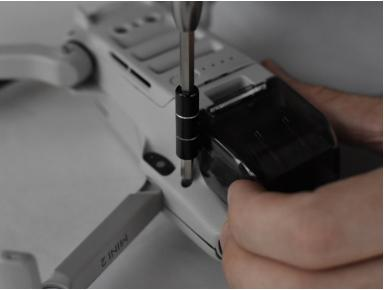
Remove the four 5 mm J000 screws near each propeller arm.
