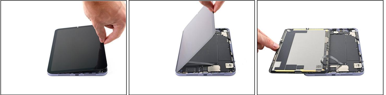
ⓘ If there's still resistance around the edges of the screen, use an opening pick to cut the adhesive again.
