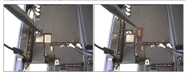
• Use the tip of a spudger to pry up and disconnect the power button board's press connector.
