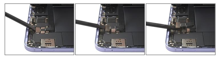
• Use the flat end of a spudger to pry up and disconnect the display cable's two press connectors secured to the frame.
