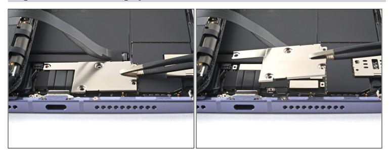
• Use tweezers, or your fingers, to remove the display cable bracket from the frame.
