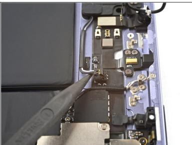
Use the point of spudger to pry up and disconnect the top speaker's cable.
