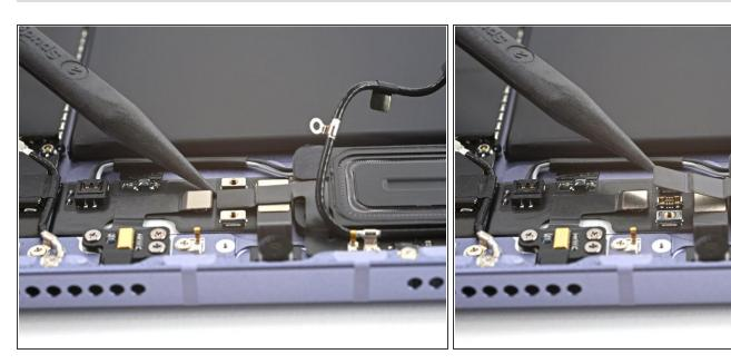
Use a spudger to pry up and disconnect the volume button board's press connector secured to the frame.
