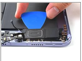
Slice along the perimeter of the top speaker to separate the adhesive.
