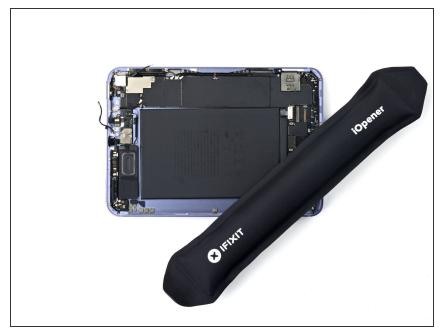
Apply a <u>heated iOpener</u> to the bottom-left edge of the device to loosen the bottom speaker's adhesive.
