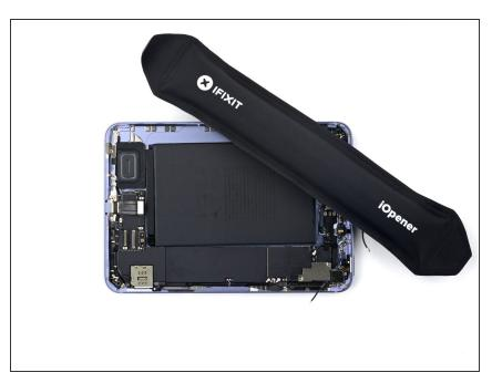
Apply a <u>heated iOpener</u> to the topleft edge of the device for 90 seconds to loosen the top speaker's adhesive.
