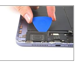
Slice along the perimeter of the bottom speaker to separate the adhesive.
