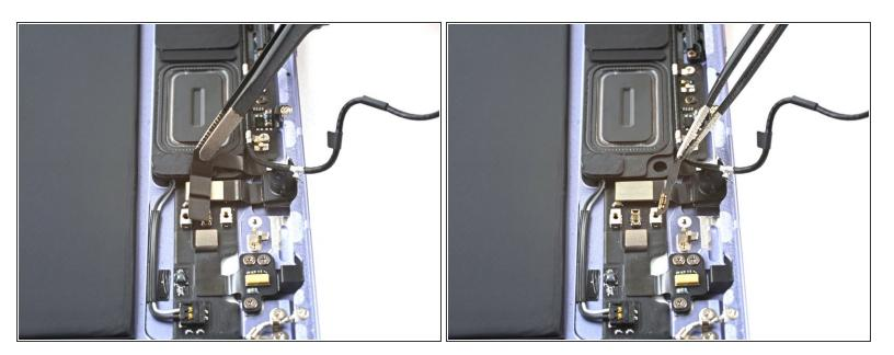
• Use tweezers, or your fingers, to peel back the volume button board's cable from the top speaker.
