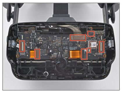
Note the seven cables that must be disconnected in the following steps before the motherboard can be removed.
