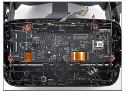
Use a T5 Torx screwdriver to remove the five 6.0 mm screws securing the motherboard to the headset.
