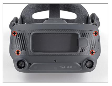
Use a T5 Torx screwdriver to remove the four 5.4 mm screws securing the motherboard cover to the headset.
