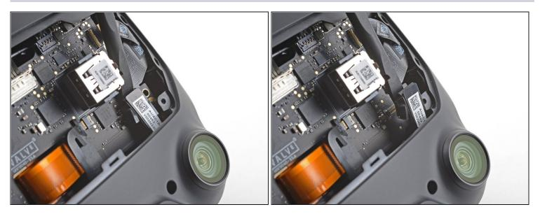
• Use the flat end of a spudger to disconnect the press connector from the bottom-right corner of the motherboard.
