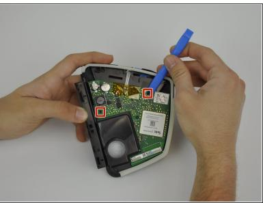
Push in the clips which secure the board to the side panel with the plastic opening tool.
