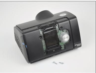
Unscrew and remove the two 11.8 mm TR10 Torx screws that were revealed from the face plate being removed.
