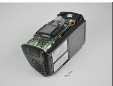
Unscrew and remove the two 11.8 mm TR10 Torx screws from the bottom of the device.
