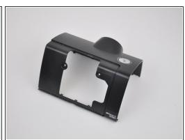
Remove the top cover from the rest of the device.
