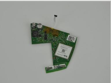
Remove the wireless communication board from the side panel.
