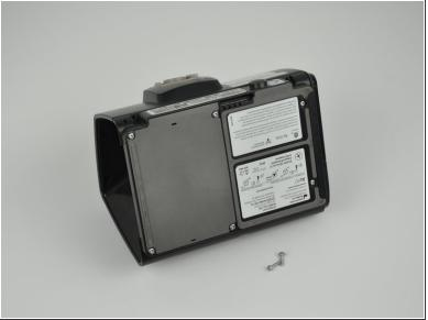
Unscrew and remove the two 11.8 mm TR10 Torx screws from the bottom of the device.
