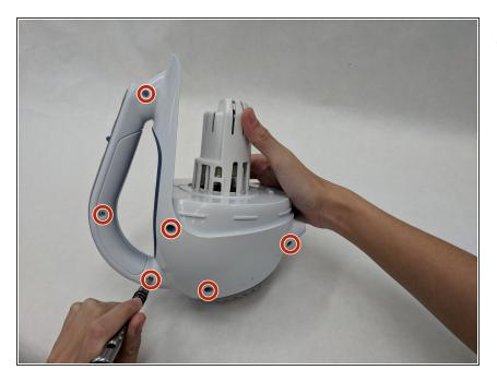
Hold the vacuum base firmly and remove all six exterior 20 mm
