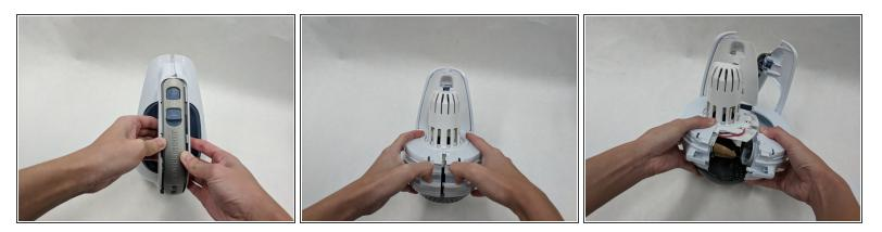
• Carefully and gently pull the two halves of the vacuum apart.
