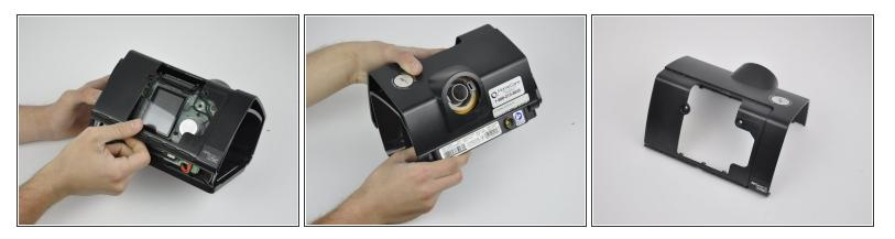
• Remove the top cover from the rest of the device.
