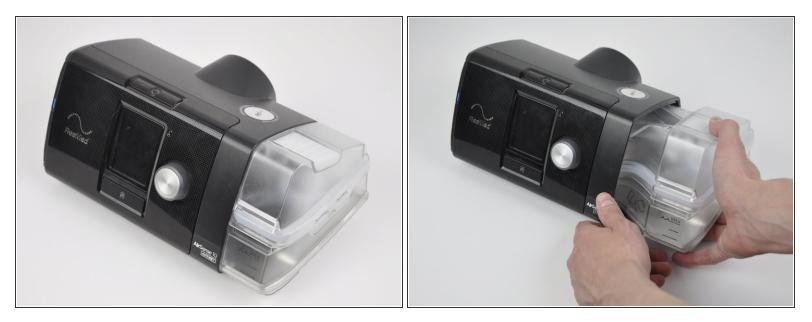
• Remove the water tub by gently pulling it out.
