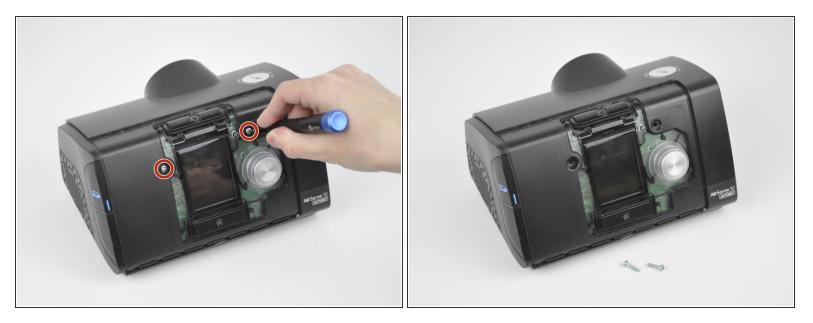
Unscrew and remove the two 11.8 mm TR10 Torx screws that were revealed from the face plate being removed.
