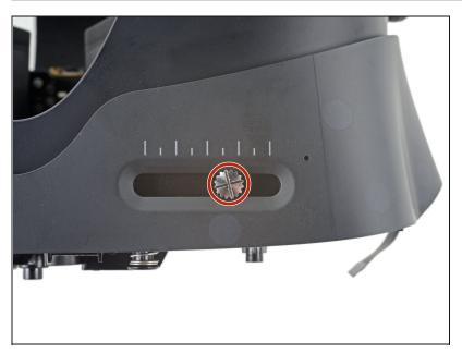
Use a 2.5 mm (3/32 in) flathead screwdriver to remove the 6.5 mm IPD screw from the headset.
