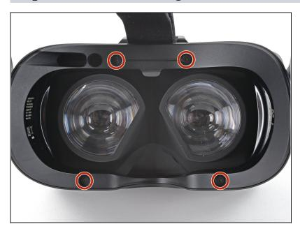
Use a T5 Torx screwdriver to remove the four 6.0 mm screws securing the face gasket bezel to the headset.
