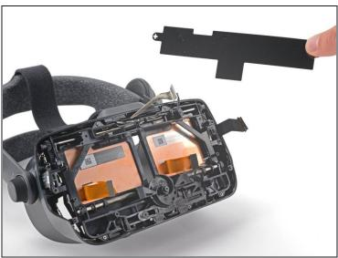
• Lift the motherboard shield off of the two cross-shaped alignment pegs.
