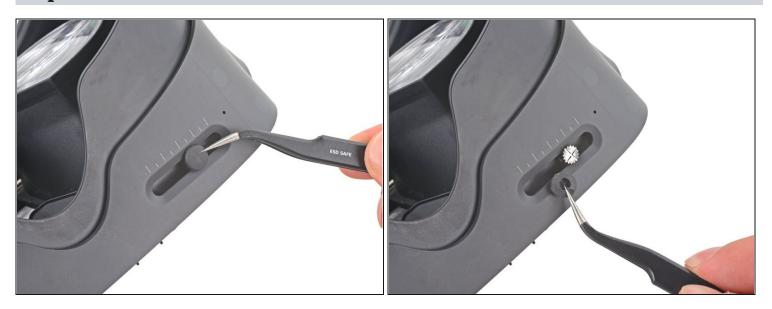
• Use your tweezers to remove the rubber boot covering the IPD adjustment screw.
