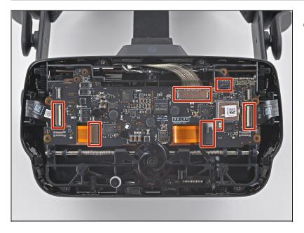
Note the seven cables that must be disconnected in the following steps before the motherboard can be removed.
