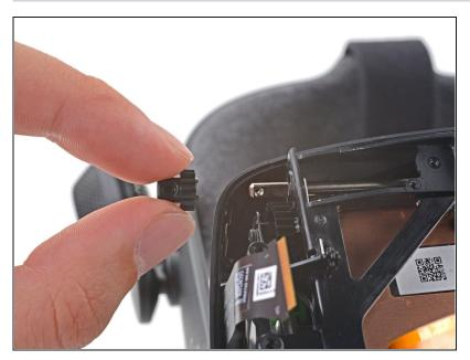
• Remove the left end gear from the eye tube rail.
