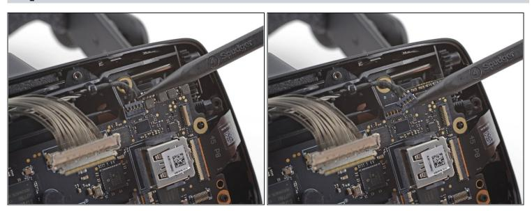
• Use the pointed end of a spudger to gently disconnect the bundled cable connector from the top-right corner of the motherboard.
