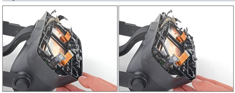
With the midframe loose, slide the case towards the back of the headset to expose the eye tube rails.
