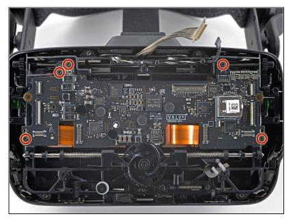
Use a T5 Torx screwdriver to remove the five 6.0 mm screws securing the motherboard to the headset.
