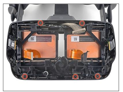
Use a T5 Torx screwdriver to remove the five 4.5 mm screws securing the midframe.
