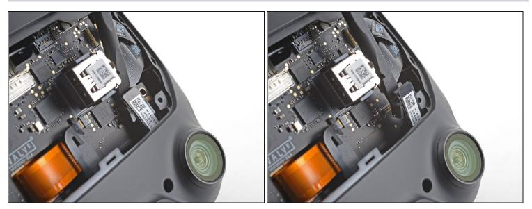
• Use the flat end of a spudger to disconnect the press connector from the bottom-right corner of the motherboard.
