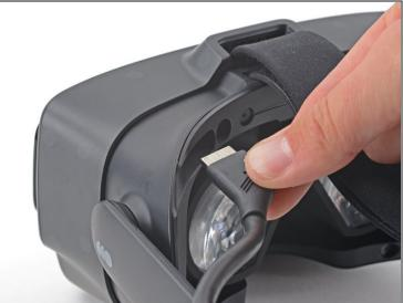
• Pull the tether cable straight back out of the headset.
