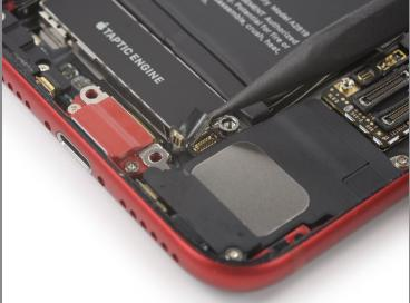
• Use the pointed end of a spudger to disconnect the Taptic Engine by prying the connector straight up from its socket.
