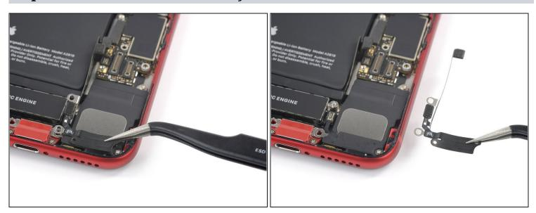
• Use a pair of tweezers to remove the Wi-Fi diversity antenna.
