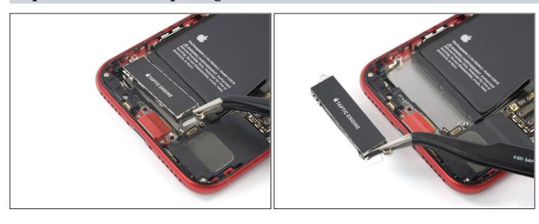
Use a pair of tweezers to carefully remove the Taptic Engine.
