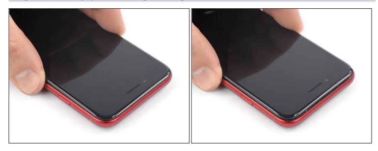
• Slide the display assembly slightly down in direction of the charging port to disengage the clips holding it to the rear case.
