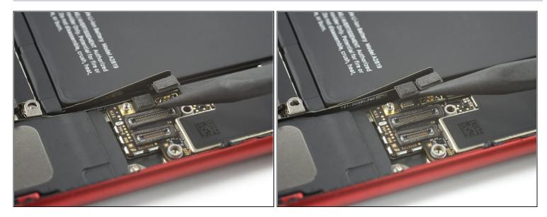
• Use the pointed end of a spudger to disconnect the Wi-Fi diversity antenna from the logic board by prying the connector straight up from its socket.
