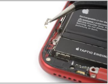
• Use a pair of tweezers to remove the grounding bracket at the left edge of the Taptic Engine.
