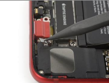
• Use the pointed end of your spudger to pry the antenna cable socket up and away from the Taptic Engine connector below.
