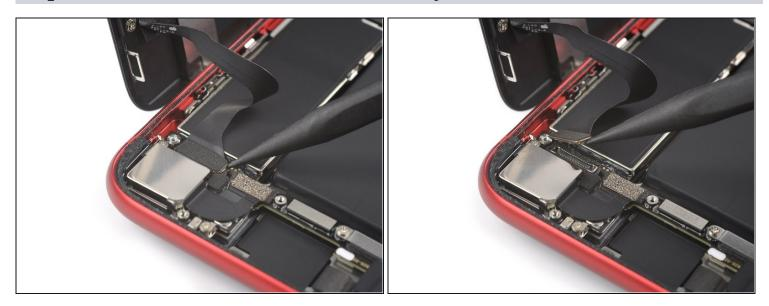
• Use the pointed end of a spudger to disconnect the front sensor assembly by prying the connector straight up from its socket.
