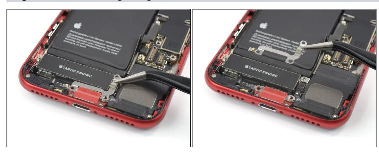
• Use a pair of tweezers to remove the Lightning connector bracket.
