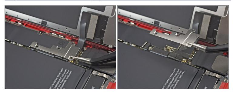
Use a pair of tweezers to carefully remove the lower display cable bracket.
