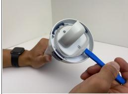
• Use a plastic opening tool to pry the clear rubber seal away from the white plastic nozzle.
